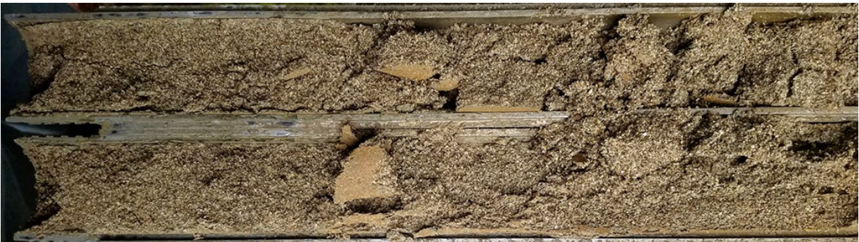
Plate 5 – Nonglacial Deposits Qpon | Medium Dense to Very dense, SAND, trace silt | PG-1, S-2 @ 5 – 6½ feet.
